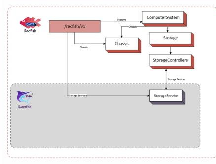
This configuration works well when the storage service is hosted by a storage resource within a computer system. An example of a Storage Service for an integrated service configuration is shown below.
