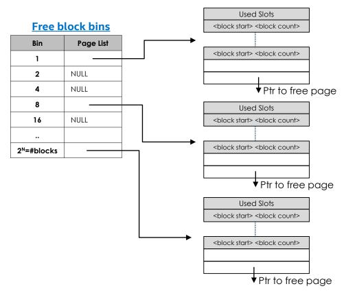
Use power of 2 binning to index into free block page pool quickly
