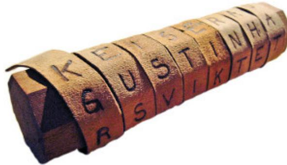
Transposition Cipher. Identical cylinders needed to align characters to recover message.
