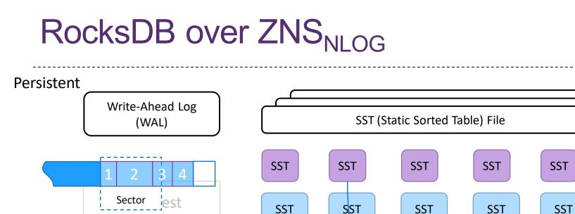
Naming the Zone eliminates filename->LBA mapping (file system), making it fast and robust.
